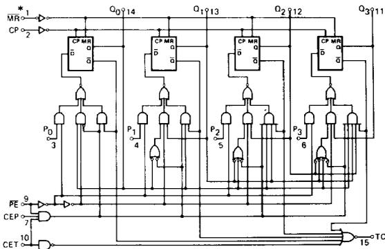
\* $\overline{MR}$  is asynchronous on the Am54S/74S161 and synchronous on the Am54S/74S163
