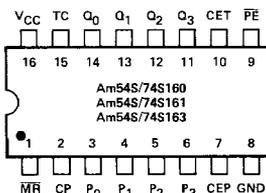
Note: Pin 1 is marked for orientation.
