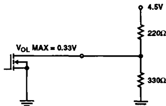
FIGURE 15B OPEN DRAIN AC/ACT TYPES EFFECTIVELY DRIVE SCSI BACKPLANE TERMINATION SCHEMES
