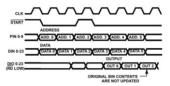
FIGURE 7. BIN ACCUMULATE TIMING
