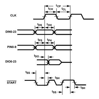
FIGURE 16. SYNCHRONOUS DATA AND CONTROL TIMING
