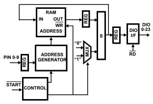
FIGURE 2. HISTOGRAM MODE BLOCK DIAGRAM
