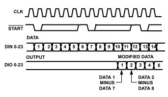
FIGURE 13. DELAY AND SUBTRACT MODE TIMING FOR ROW LENGTH OF TEN
