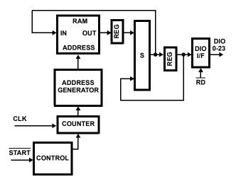
FIGURE 4. HISTOGRAM ACCUMULATE MODE BLOCK DIAGRAM
