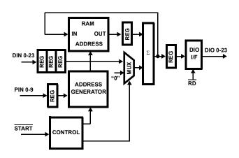
FIGURE 6. BIN ACCUMULATE BLOCK DIAGRAM
