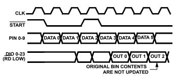
FIGURE 3. HISTOGRAM MODE TIMING
