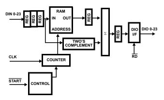
FIGURE 12. DELAY AND SUBTRACT BLOCK DIAGRAM
