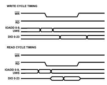
FIGURE 15. ASYNCHRONOUS 16/24 MODE TIMING
