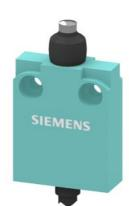
Position switch in compact design 40 mm wide with connection cable 2 m Snap-action contacts 1 NO+1 NC with rounded plunger with exterior seal
