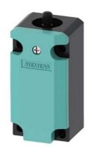
Basic switch with increased corrosion protection for position switch Metal enclosure, according to EN 50041 Device connection 1 x (M20 x 1.5) 1 NO/1 NC quick action contacts without actuator head
