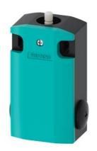
Basic switch for position switch 3SE5162 Metal enclosure XL, 56 mm wide Device connection  $3x(M20\ x\ 1.5)$  IP66/IP67 2 x (1 NO/1 NC) quick action contacts without actuator head
