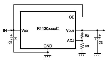
$C1\text{=}C2\text{=}0.1\mu\text{F},\,R2,\,R3\text{:}$  Refer to the Technical Notes on Output Voltage setting of C type.
