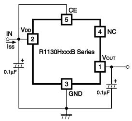
**Fig.2 Supply Current Test Circuit**
