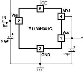
**Fig.2 Test Circuit Supply Current**
