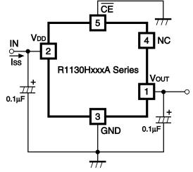
**Fig.2 Supply Current Test Circuit**
