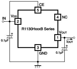
Fig.1 Standard test Circuit
