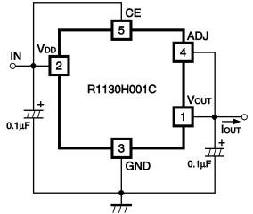
Fig.1 Standard test Circuit
