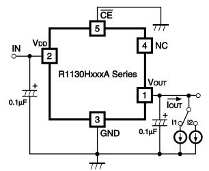
**Fig.4 Load Transient Response Test Circuit**
