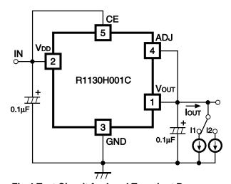
Fig.4 Test Circuit for Load Transient Response
