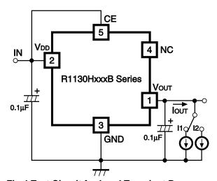
Fig.4 Test Circuit for Load Transient Response
