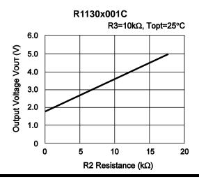
\* Adjustable Resistor Dependence of Output Voltage
