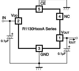
Fig.1 Standard test Circuit
