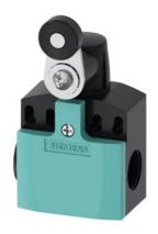
Position switch Plastic 50 mm, Increased corrosion protection Device connection 2 x (M20 x 1.5) 1 NO/1 NC snap-action contacts twist lever metal lever with plastic roller 19 mm functional at -40 °C Shock and vibration test according to EN 61373, Category 1B
