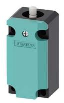
Basic switch for position switch 3SE513 Enclosure plastic according to EN 50041, 1 x (M20 x 1.5) 1 NO/1 NC slow-action contacts without actuator head
