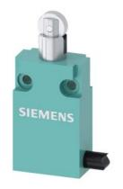
Position switch in compact design 30 mm wide with connecting cable 5 m Snap-action contacts 1 NO+1 NC with roller plunger
