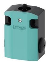
Position switch Basic switch Metal, 56 mm Increased corrosion protection Device connection 3 x (M20 x 1.5) 1 NO/2 NC slow-action contacts functional at -40  $^\circ$ C Shock and vibration test according to EN 61373, Category 1B
