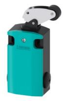
Position switch 3SE5162 Metal enclosure XL, 56 mm wide with angular roller lever Metal lever and Plastic roller 22 mm Device connection 3 x (M20 x 1.5) 2 x (1 NO/1 NC) Quick action contacts IP66/IP67
