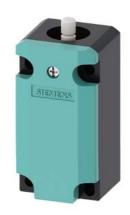
Position switch Basic switch Metal, 40 mm, according to EN 50041 Increased corrosion protection Device connection 1 x (M20 x 1.5) 1 NO/2 NC slow-action contacts functional at -40  $^{\circ}\text{C}$  Shock and vibration test according to EN 61373, Category 1B
