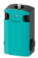
Basic switch for position switch 3SE5162 Metal enclosure XL, 56 mm wide Device connection  $3x(M20 \times 1.5)$  IP66/IP67 2 x (1 NO/2 NC) Slow-action contacts without actuator head with increased corrosion protection
