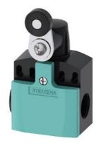
Position switch Plastic enclosure according to EN 50047, 50 mm Device connection 2 x (M20 x 1.5) 1 NO/2 NC quick action contacts twist lever right/left adjustable with plastic roller 19 mm
