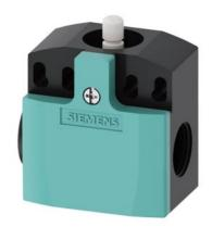
position switch plastic enclosure 50 mm, device connection 2 x (M20 x 1.5) 1 NO/1 NC quick-action contacts 2 x 2 mm contact gap rounded plunger
