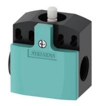
position switch with increased corrosion protection plastic enclosure 50 mm, device connection 2 x (M20 x 1.5) 1 NO/1 NC slow-action contacts, rounded plunger
