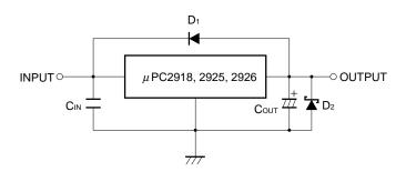
$C_{IN}: 0.1~\mu F$  or higher. Be sure to connect  $C_{IN}$  to prevent parasitic oscillation. Set this value according to the length of the line between the regulator and the INPUT pin. Use of a film capacitor or other capacitor with first-rate voltage and temperature characteristics is recommended. If using a laminated ceramic capacitor, it is necessary to ensure that  $C_{IN}$  is  $0.1~\mu F$  or higher for the voltage and temperature range to be used.
