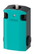
Basic switch for position switch 3SE5162 Metal enclosure XL, 56 mm wide Device connection  $3x(M20\ x\ 1.5)$  IP66/IP67 2 x (1 NO/1 NC) quick action contacts without actuator head with increased corrosion protection
