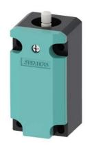
Basic switch with increased corrosion protection for position switch 3SE513 Enclosure plastic according to EN 50041 Device connection 1 x (M20 x 1.5) 1 NO/2 NC slow-action contacts without actuator head
