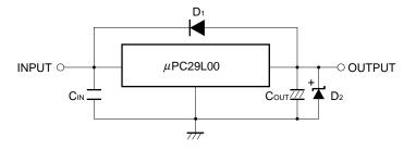
C<sub>IN</sub> : 0.1 to 0.47  $\mu$ F. C<sub>OUT</sub> : More than 10  $\mu$ F. D<sub>1</sub> : Need for Vo > V<sub>IN</sub>. D<sub>2</sub> : Need for Vo < GND.
