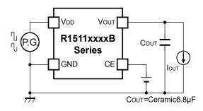
R1511xxxxB Test Circuit for Ripple Rejection and Regulator Input Transient Response
