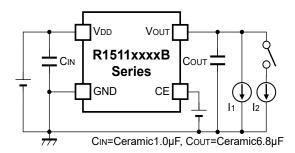
R1511xxxxB Test Circuit for Load Transient Response
