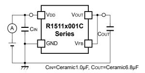
R1511x001C Test Circuit for Supply Current
