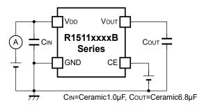
R1511xxxxB Test Circuit for Supply Current
