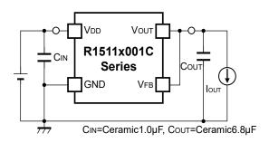
R1511x001C Basic Test Circuit
