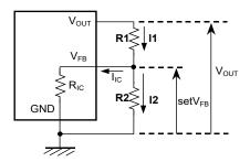
**Output Voltage Adjustment Using External Divider Resistors**
