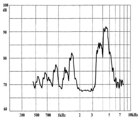
**Note:** Input Voltage 10Vp-p square wave Distance 30 cm
