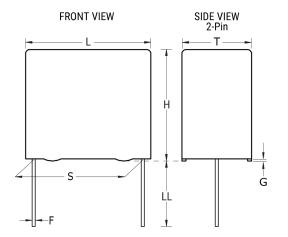
**General Information** Series PFR/F411 Dielectric Film/Foil Polypropylene Style Radial Features Pulse RoHS Yes Lead Wire Leads AEC-Q200 No Typical Component 0.362 g Weight An Operating Temperature Up To +105C Is Miscellaneous Allowed Under Certain Conditions. Please Consult KEMET For Details.
