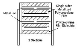
Film Capacitors – General Purpose, Pulse and DC Transient Suppression PHE448 Polypropylene Film/Foil, Radial
