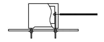
Temperature monitored inside the capacitor.
