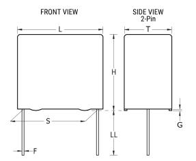
**General Information** Series PFR/F411 Dielectric Film/Foil Polypropylene Style Radial Features Pulse RoHS Yes Lead Wire Leads AEC-Q200 No Typical Component 0.345 g Weight An Operating Temperature Up To +105C Is Miscellaneous Allowed Under Certain Conditions. Please Consult KEMET For Details.
