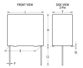
**General Information** Series PFR/F411 Dielectric Film/Foil Polypropylene Style Radial Features Pulse RoHS Yes Lead Wire Leads AEC-Q200 No Typical Component 0.374 g Weight An Operating Temperature Up To +105C Is Miscellaneous Allowed Under Certain Conditions. Please Consult KEMET For Details.
