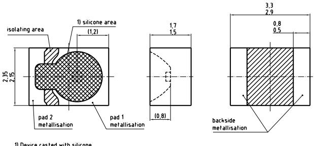
Device casted with silicone. Avoid mechanical stress on silicone surface.
