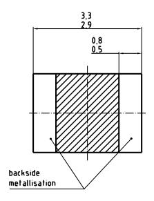
1) Device casted with silicone. Avoid mechanical stress on silicone surface.
