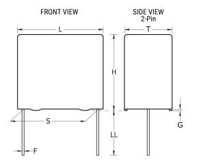
**General Information** Series PFR/F411 Dielectric Film/Foil Polypropylene Style Radial Features Pulse RoHS Yes Lead Wire Leads AEC-Q200 No Typical Component 0.37 g Weight An Operating Temperature Up To +105C Is Miscellaneous Allowed Under Certain Conditions. Please Consult KEMET For Details.
