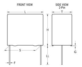
**General Information** Series PFR/F411 Dielectric Film/Foil Polypropylene Style Radial Features Pulse RoHS Yes Lead Wire Leads AEC-Q200 No Typical Component 0.36 g Weight An Operating Temperature Up To +105C Is Miscellaneous Allowed Under Certain Conditions. Please Consult KEMET For Details.
