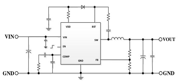
Note: When using a solid or ceramic input Cap, It is recommended to parallel a TVS diode.
