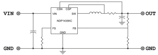
Note: When using a solid or ceramic input Cap, It is recommended to parallel a TVS diode.
