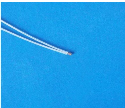
Figure 1.2 The physical photo of ATH10KR8B3404KT65
