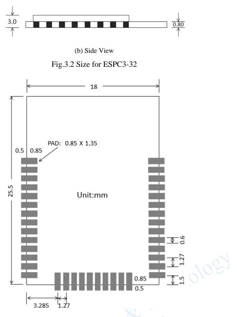
Fig. 3.3 PCB Layout for ESPC3-32
