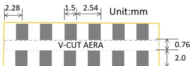
Fig. 3.3 PCB Layout for ESP-M4
