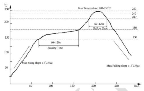
Fig.7.1 Recommended Reflow Profile
