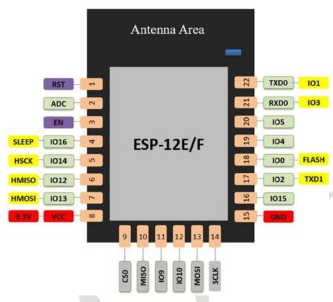
Fig. 2.1 ESP-12F Pins Definition
