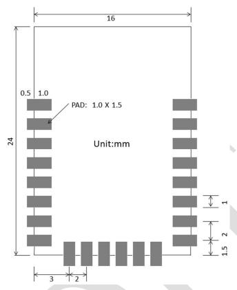
Fig. 3.3 PCB Layout for ESP-12F Table 3.1 Size for ESP-12F
