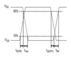
Figure D. Resistive Switching Waveforms
