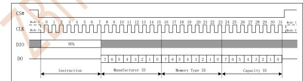
Figure 7.31a Read JEDEC ID(SPI Mode)
