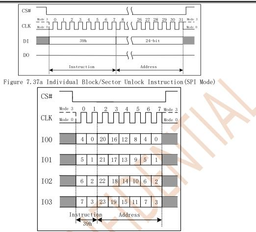
Figure 7.37b Individual Block/Sector Unlock Instruction (QPI Mode)
