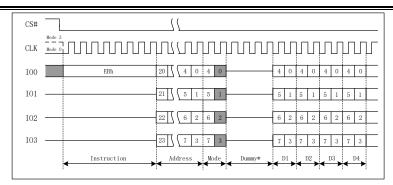
Figure 7.19a Fast Read Quad I/O Instruction(Initial command or previous  $M5-4 \neq 10$ )
