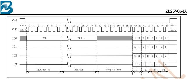
Figure 7.16 Fast Read Quad Output Instruction
