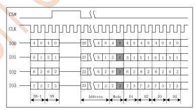
Figure 7.24 Octal Word Read Quad I/O Instruction(Initial command or previous M5-4 =10)
