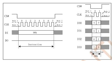
Figure 7.40 Global Block Lock Instruction (SPI or QPI Mode)
