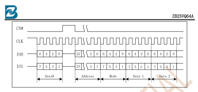
Figure 7.18 Fast Read Dual I/O Instruction (Initial command or previous M5-4=10)
