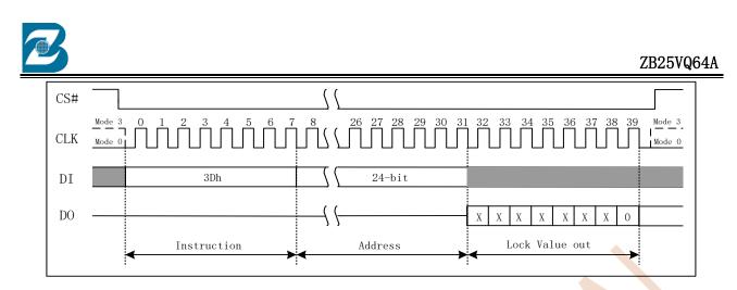
Figure 7.38a Read Block Lock Instruction(SPI Mode)
