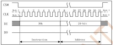
Figure 7.36a Individual Block/Sector Lock Instruction(SPI Mode)
