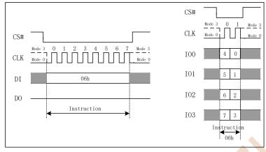
Figure 7.2 Write Enable Instruction (SPI or QPI Mode)
