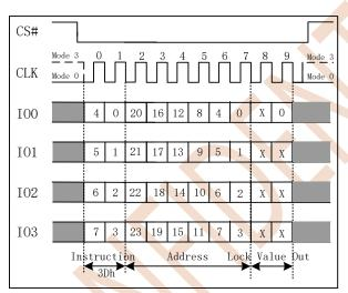
Figure 7.38b Read Block Lock Instruction(QPI Mode)
