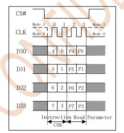
Figure 7.44 Set Read Parameters Instruction (QPI Mode only)
