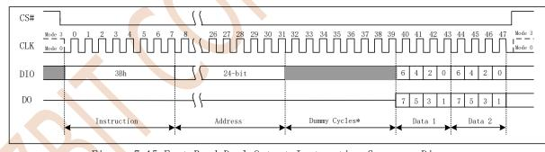
Figure 7.15 Fast Read Dual Output Instruction Sequence Diagram
