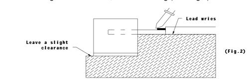
Regarding solution in the tinning oven for product-tinning, compound sub-solution made of tin & copper and sliver is proposed with the temperature of Celsius 260. The proportion of the alloyed solution is tin 95.5: copper 3.5: silver 0.5 by percentage. The time of tinning is constantly 3 seconds.
