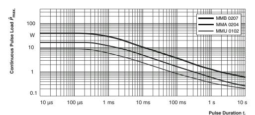
Maximum pulse load, continuous pulses; applicable if  $\bar{P} \leq P\left(\vartheta_{amb}\right)$  and  $\hat{U} \leq \hat{U}_{max}$ ; for permissible resistance change equivalent to 8000 h operation
