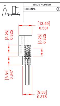
DIALLYL PTHYHALATE, UL94V-0 CONTACT MATERIAL: COPPER ALLOY CONTACT PLATING: GOLD PLATING OVER NICKEL 6 TO 16 Oz (0.56 TO 4.45N) PER CONTACT INSERTION FORCE: WITHDRAWAL FORCE: 6 TO 16 Oz (0.56 TO 4.45N) PER CONTACT
