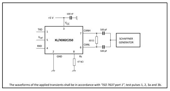
Figure 6-6. Test circuit for transients
