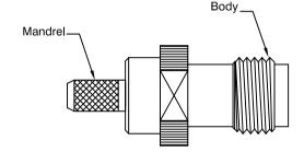
3) Insert the contact into the body and ensure that the contact captivates. Make sure that the braid is on the outside of the mandrel. Slide the ferrule over the braid until the ferrule butts up against the body. Crimp the ferrule using the correct tool for the connector.
