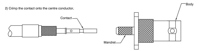
3) Insert the contact into the body and ensure that it captivates. Make sure that the braid is on the outside of the mandrel. Slide the ferrule over the braid until the ferrule butts up against the body. Crimp the ferrule using the correct tool for the connector.
