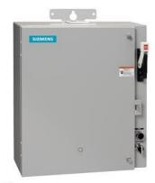
Pump control panel, Size 3 1/2, Three phase full voltage, Solid-state overload relay, OLR amp range 50-200A, 24VAC 50-60Hz coil, Standard type contactor, 125A circuit breaker, HOA Sel Sw. <(>&<)> Start P.B., Enclosure NEMA type 3/3R, Weather proof outdoor use
