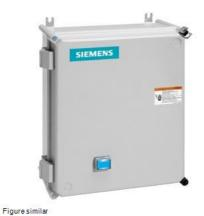
Non-reversing motor starter, Size 4, Three phase full voltage, Solid-state overload relay, OLR amp range 50-200A, 208VAC 60Hz coil, Non-combination type, Enclosure type 4X fiberglass, Water/dust tight noncorrosive, Standard width enclosure
