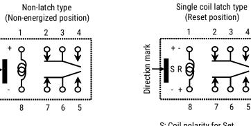
S: Coil polarity for Set R: Coil polarity for Reset
