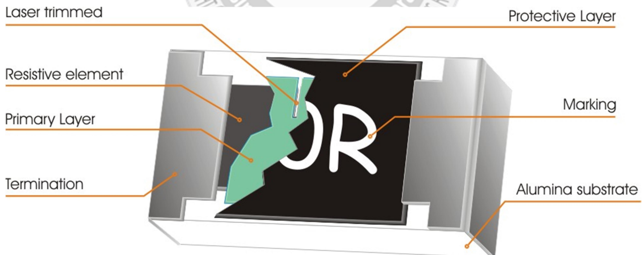
Fig 1. Construction of Chip-R
